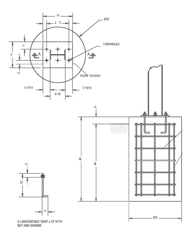
The above drawing is a representation of typical construction details and is not intended to be used without consulting with eNoise Control's Engineering Department for your specific use.
