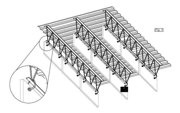
Baffle Suspension with Bar Joist and Deck Construction
